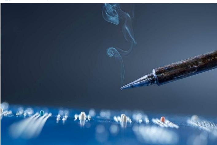
In most soldering methods, the first step involves pre-cleaning and deoxidation of surface oxides, usually involving a liquid flux material. While this method gets the job done, fusing of traditional lead-tin solders leaves flux residue that has to be removed, often by an expensive, environmentally hazardous cleaning method.
